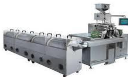
Fig 7. Soft gelatin capsule drying machine
